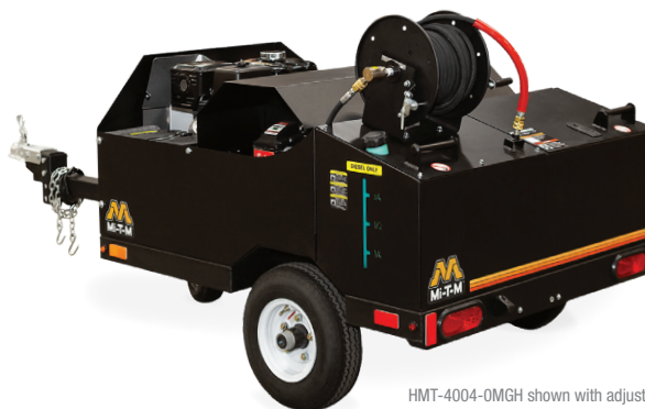
HMT-4004-OMGH shown with adjustable trailer coupler hitch, TX-0010, high pressure hose reel, TX-0020 and 100-foot hose, 15-0161
