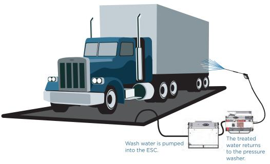
vacuum system with auto pump out. The pre-filtered waste stream will enter the easiest and simplest to maintain system ever designed for water treatment.
